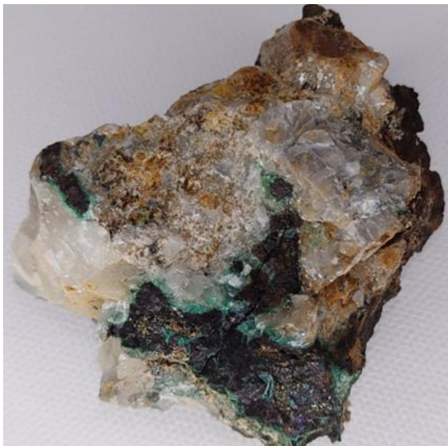
Figure 6 - Sample R22CR0160, coarsely crystalline marble outcrop at Clifford. Coarse masses of chalcopyrite and bornite with development of malachite rims are prominent. Approximate scale: 6cm across.
