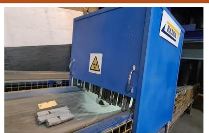
Figure 1 Rados overbelt XRF analyser testing Coda's Emmie Bluff core at a Rados facility in South Africa. This work was undertaken as part of phase 1, prior to in-field trials.
