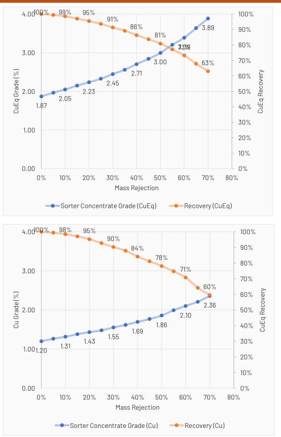
Figure 2 Ore sorter recovery and grade improvement on a copper equivalent (upper) and copper (lower) basis from simulated diluted ore at a simulated mined head grade of 1.87% CuEq, 1.20% Cu.
