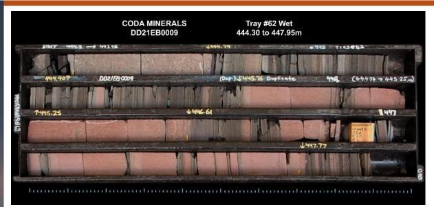
Figure 3 Sandy interbeds (pink) within mineralised shale (black/grey) represent internal dilution, a prime candidate for ore sorting.
