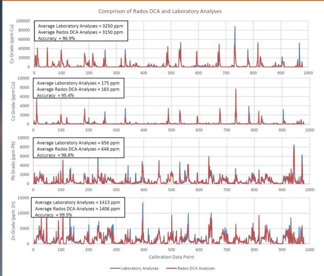
Figure 4 Results of scanning after calibration against assay data. To estimate the grade of cobalt in the drill core samples, Rados's XRF+ sensor incorporated machine learning algorithms that utilized the patterns using the full XRF spectrum. This feature contributed to accurately determining the cobalt (Co) grade, successfully overcoming the challenges posed by inter-element interferences commonly encountered in conventional XRF analysis, in particular those caused by iron (Fe) and nickel (Ni).
