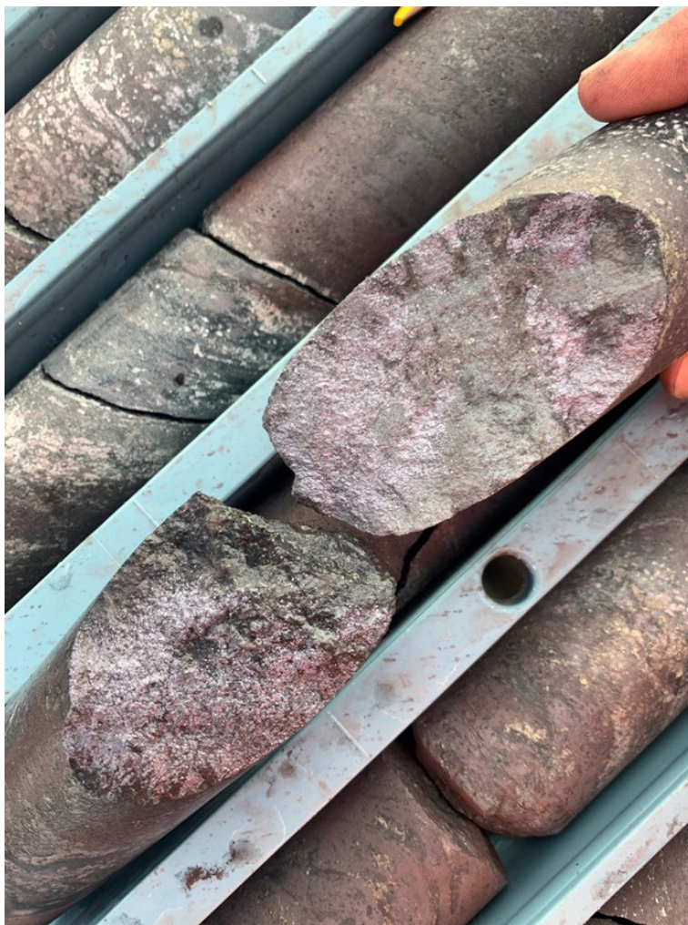
Figure 7 (left): Fracture filling molybdenite, approx. 929.5m.
