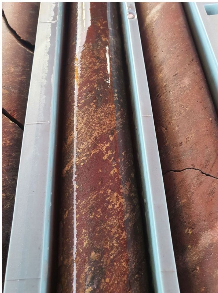
Figure 5 (left): Bedding parallel blebs and aggregates in red earth haematite altered sediments, approx. 925m.
