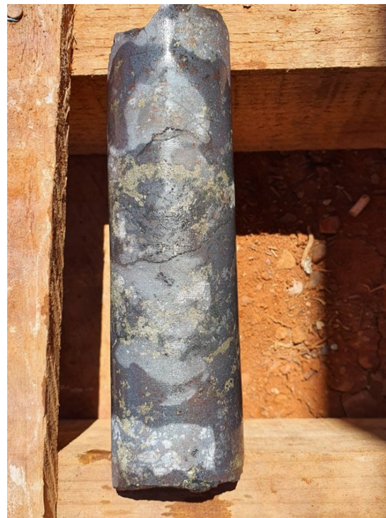
Figure 3 (left): Shallowest encountered mineralisation in wedge hole 2W4: Blebby chalcopyrite at approx. 862m, part of approx. 1.5m of similar mineralisation.
