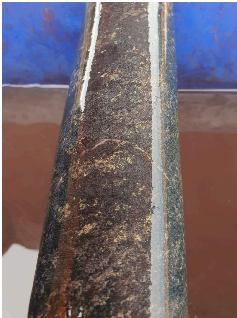
Figure 9 (left): Blebby/disseminated chalcopyrite in strongly haematised core, approx. 948m.
