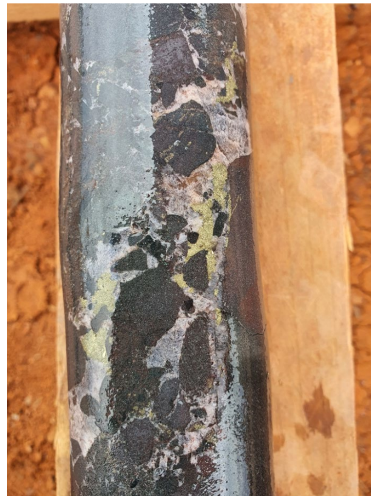
Figure 9 (left): Blebby/disseminated chalcopyrite in strongly haematised core, approx. 948m.
