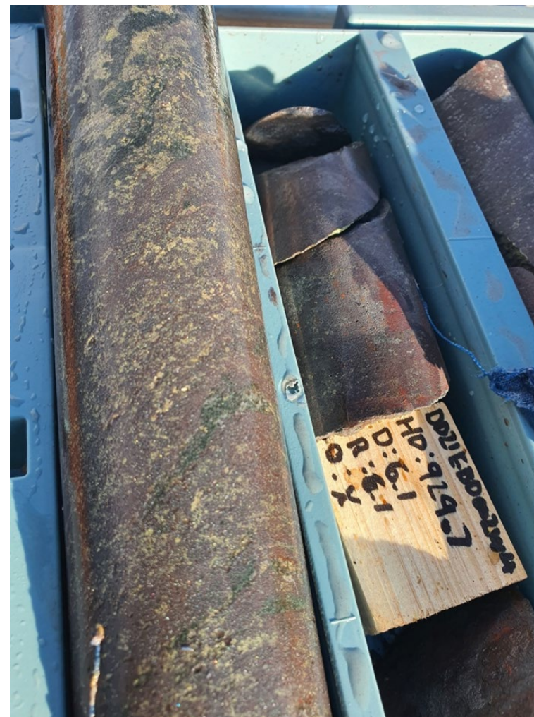
Figure 5 (left): Bedding parallel blebs and aggregates in red earth haematite altered sediments, approx. 925m.
