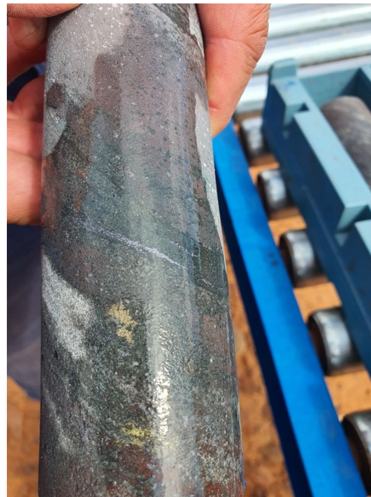
Figure 7 (left): Fracture filling molybdenite, approx. 929.5m.
