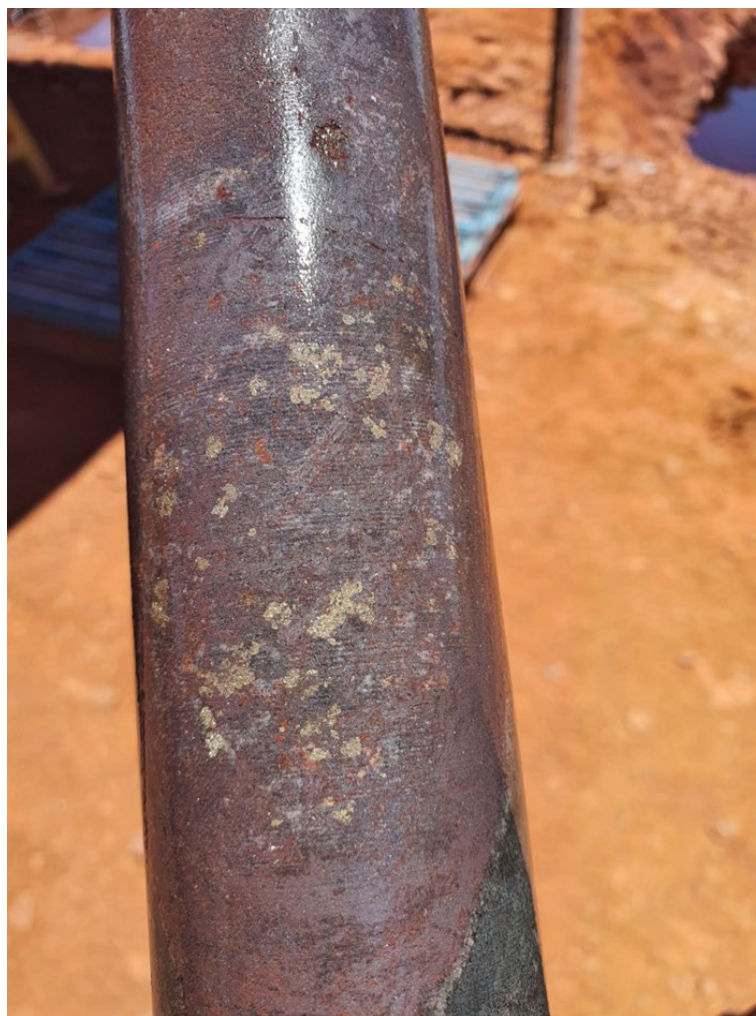
Figure 3 (left): Shallowest encountered mineralisation in wedge hole 2W4: Blebby chalcopyrite at approx. 862m, part of approx. 1.5m of similar mineralisation.
