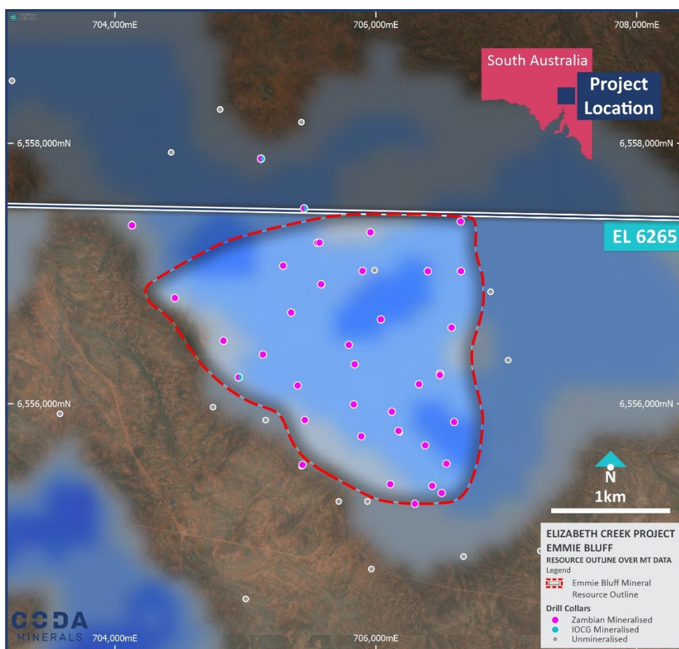
Figure 6 3D inverted ground magnetotelluric data (originally collected 2010, reprocessed 2021) showing continuity of low resistivity anomalism to the east of the Emmie Bluff Mineral Resource. The western, fault bounded margin of the basin is well defined by contrast.
