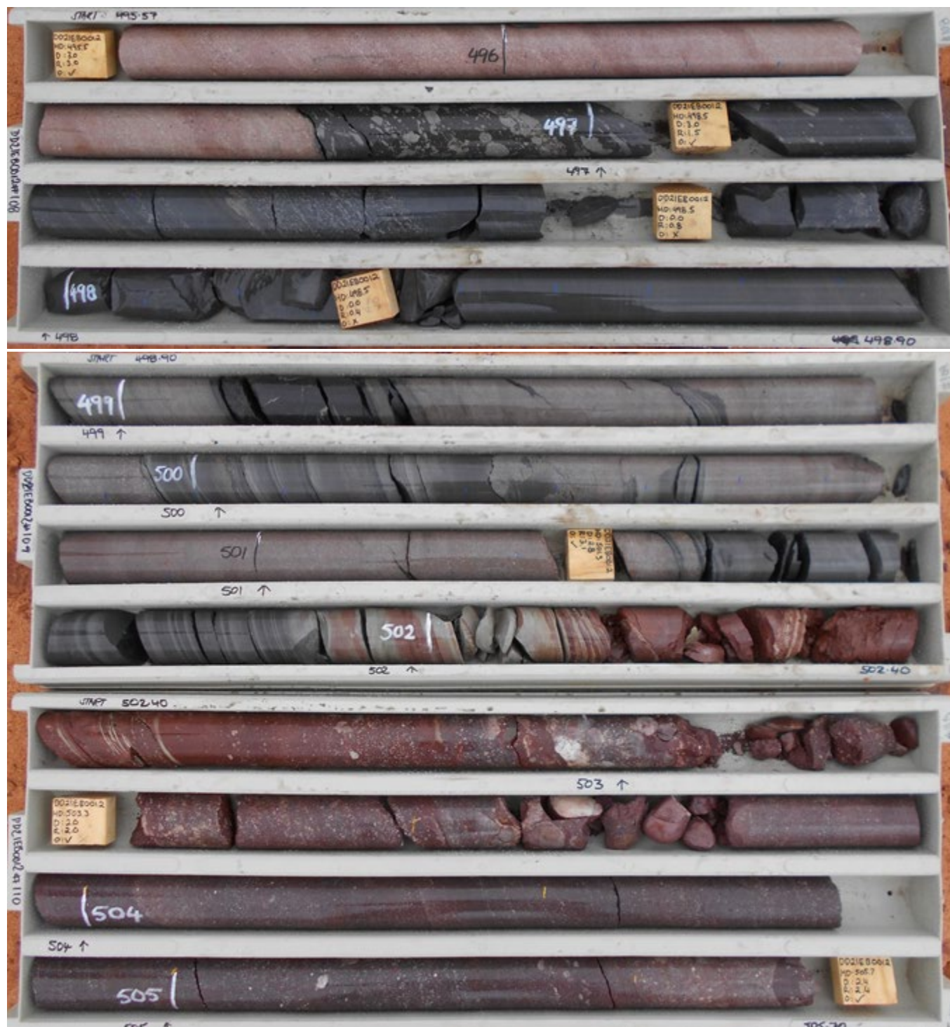
Figure 5 Core photos showing the transition from Whyalla Sandstone to Tapley Hill Formation and into Pandurra Formation, encompassing the mineralised intersections in hole DD21EB0012. Mineralisation is closely tied to the presence of reducing black shale and negatively correlated with lower carbon sands beds, which are easily discriminated.
