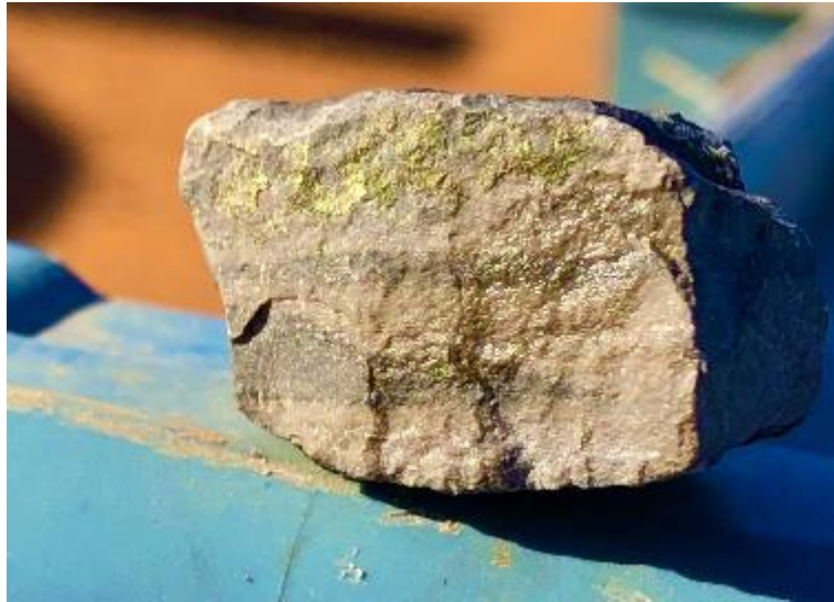
Figure 5 Mineralised RC chip from RC21MG140020. Rock chip is approx. 15mm across.
