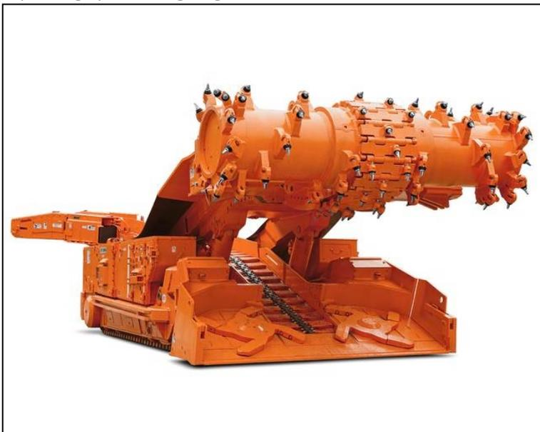
Figure 12: Development 12HM27 Continuous Miner, Komatsu
