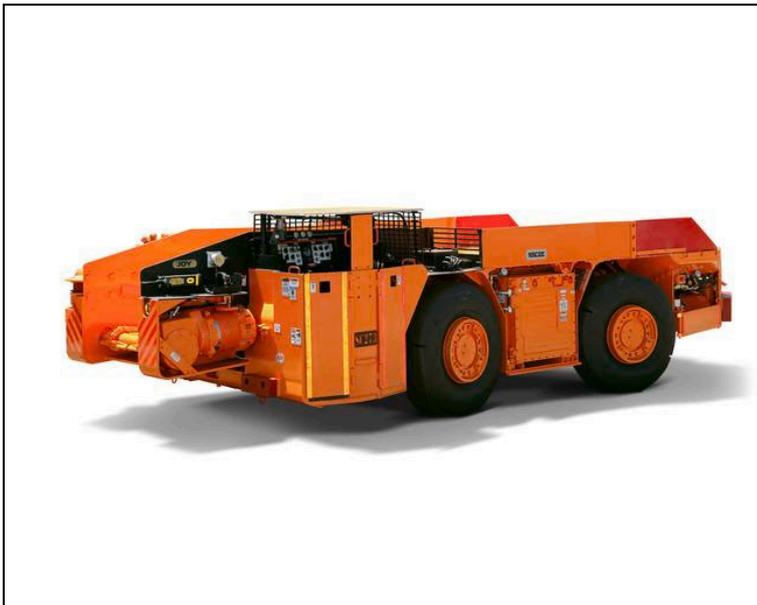
Figure 14: Shuttle car 10SC32, Komatsu
