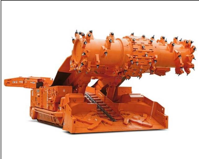
Figure 13: Production 12HM36 Continuous Miner, Komatsu
