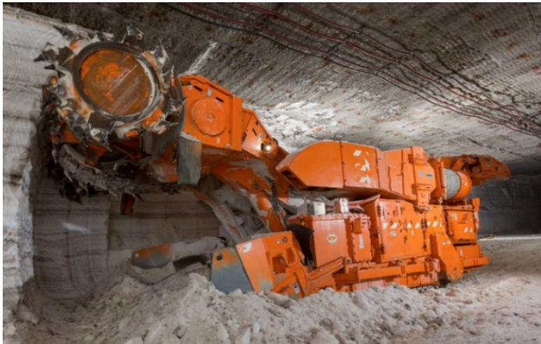
Mechanical cutting using a continuous miner at Emmie Bluff is an attractive alternative to drill-and-blast for numerous reasons – resulting in a lower operating cost, higher productivity, an improved geotechnical tolerance and the ability to mine at narrower and more precise tolerances, allowing for the exploitation of even relatively narrow mineralised lodes with minimal dilution.
