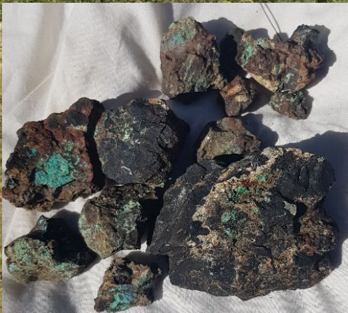
Sample R21CR0143, bleached and altered Corella Fm. Rebound prospect. 2.74g/t Au, 156g/t Ag, 9.15% Cu
