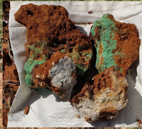
Sample R21CR0310, ferruginous gossan/quartz vein in Corella Fm, Clear Waters prospect. 0.3g/t Au, 4g/t Ag, 22.89% Cu
