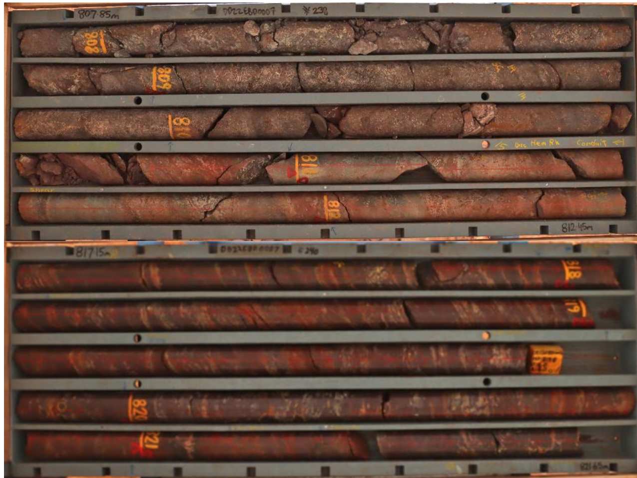
Figure 4 Upper tray (807.85m to 812.45m) of EBD7 drill core: Discordant haematite, interpreted as a fracture filling (conduit) material, likely associated with proximal bornite/chalcocite dominated mineralisation. Lower tray (817.15m to 821.65m): Mineralised Wallaroo Group sediments, strongly haematised. Note the preservation of remnant bedded texture in contrast with the conduit material.
