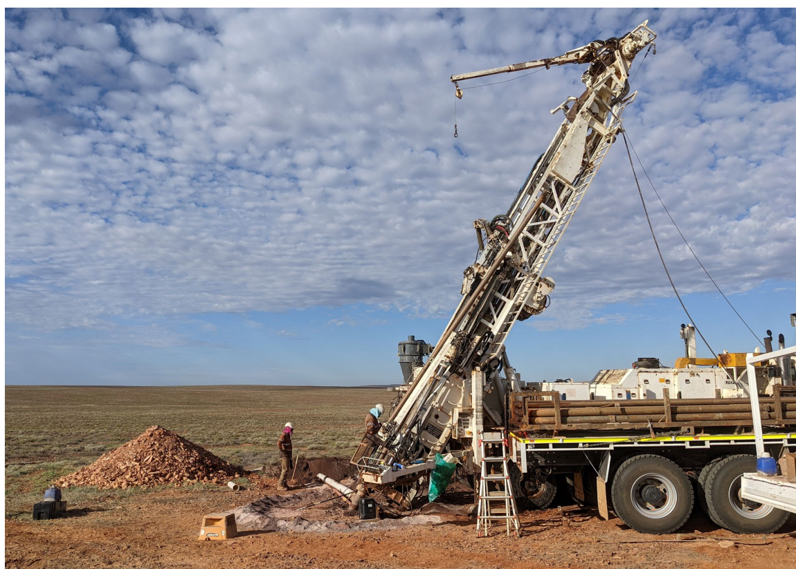
Figure 5 Commencement of RC precollar at Emmie East Zambian-style Cu-Co-Ag prospect.
