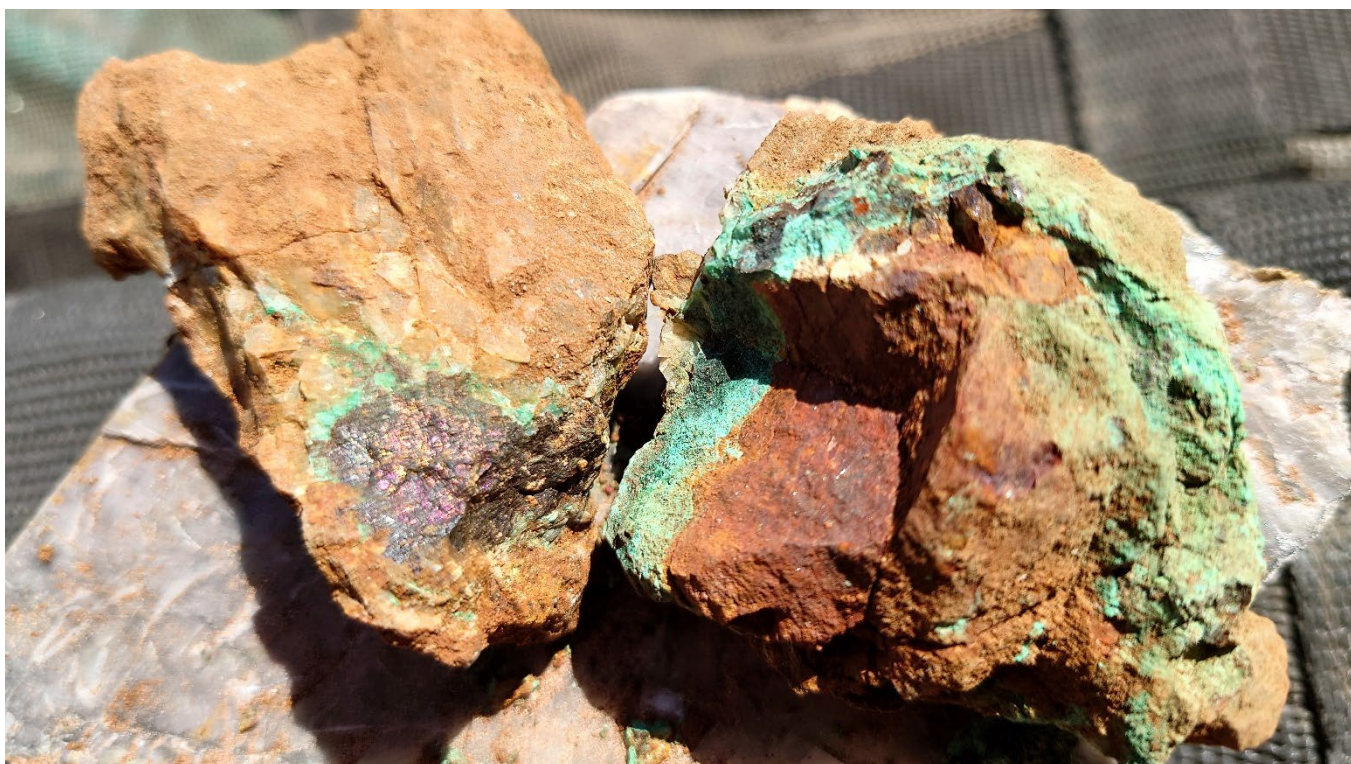
Figure 3 Grab sample of mineralised quartz-calcite vein exposed in the drill pad of RC22CR0017 and RC22CR0018 at Copper Weed South. The sample contains coarse masses of chalcopyrite (3%) with minor bornite (1%) and trace covellite (0.1%), with development of malachite (10%) as rimming to the sulphide masses.
