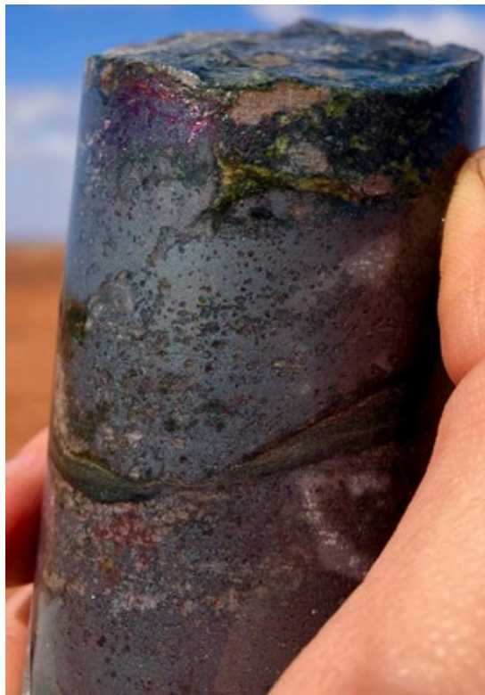
Figure 3. Intense steely haematite alteration with bornite and possible covellite at 818m in DD21EB0001W2.
