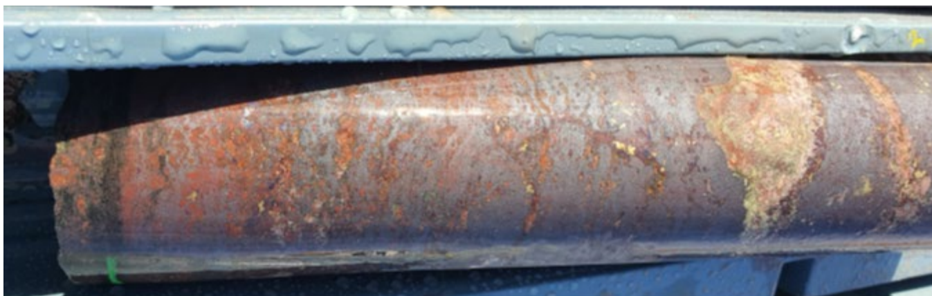
Figure 10 Intensely haematite altered metasediment breccia, 821m DD21EB0018W1. Minor sulphide blebs of bornite and chalcopyrite.
