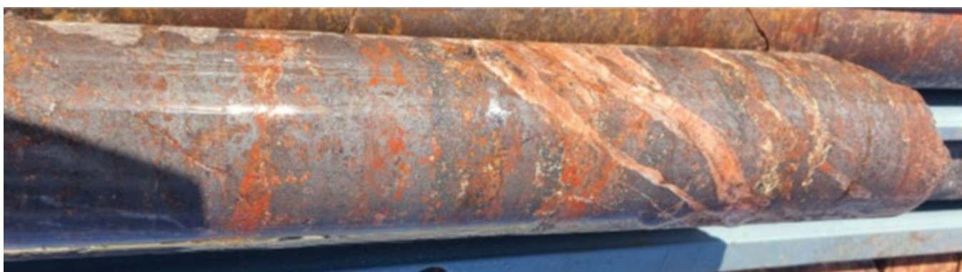
Figure 9 Haematite altered chalcoite/bornite zone, 809.5m DD21EB0018W1. Veining is primarily baryte.
