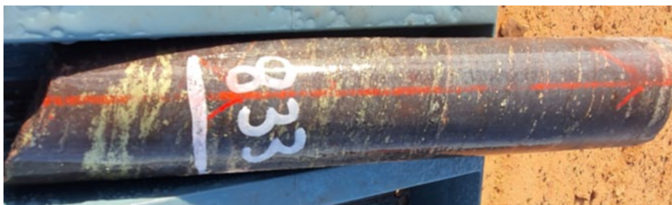
Figure 2. Intense sulphide and haematite alteration in DD21EB0001W1 at 833m. Sulphides are dominated by chalcopyrite and have deposited roughly aligned with remnant sedimentary structures (bedding).
