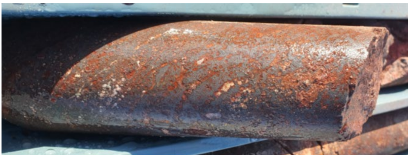
Figure 8 Close up showing remnant sedimentary structures preserved in remnant haematite "cap", DD21EB0018W1, 708.3m
