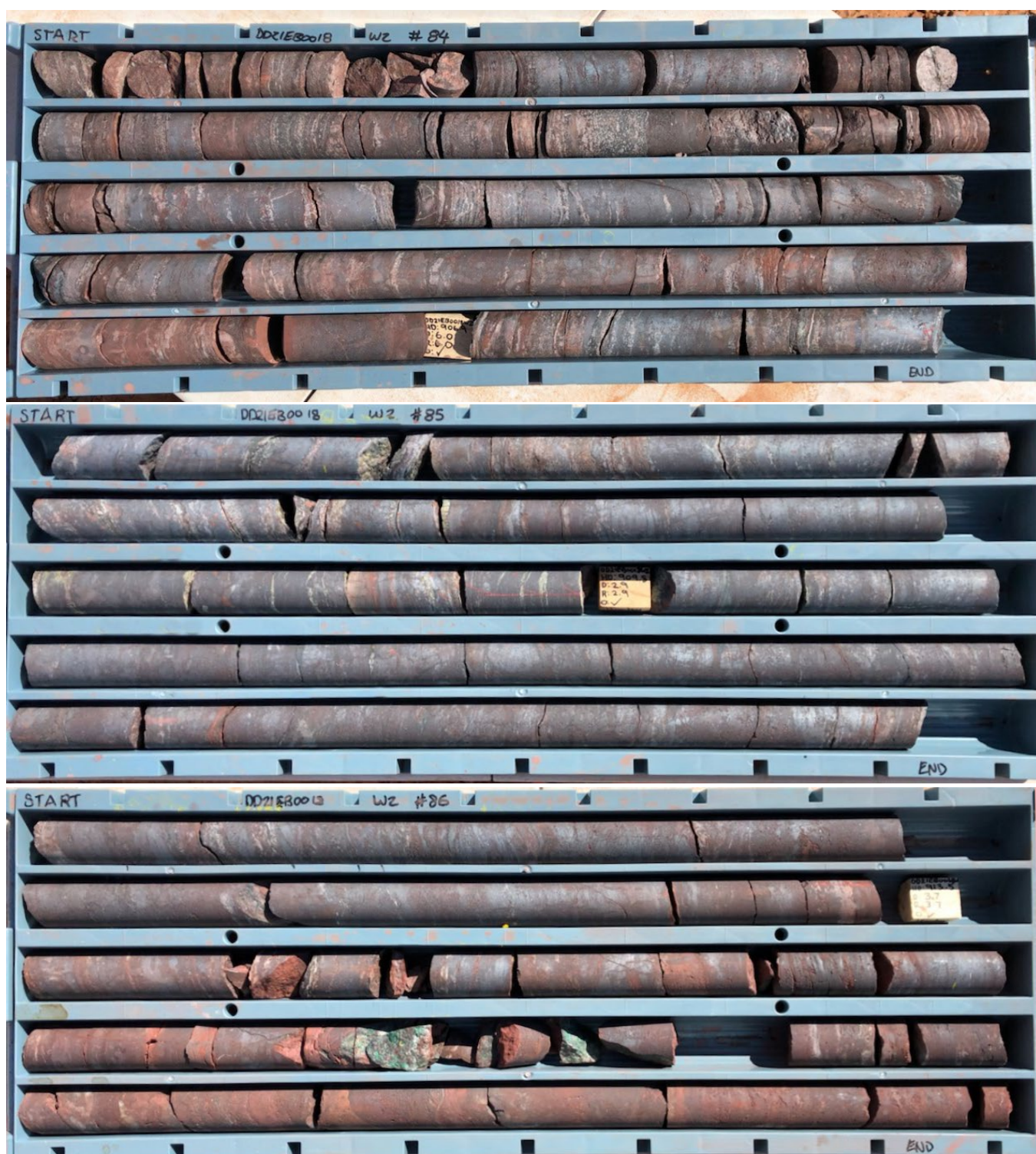
Figure 12 Lower mineralised horizon from DD21EB0018W2. Disseminated bornite is not readily visible in images but is easily discerned in hand sample. Presence of copper has been confirmed by handheld XRF. Note alteration on fracture surfaces – field geologists have identified as malachite, interpreted as a secondary alteration product following post-mineralising fluid flow events. It is very unusual to see malachite, a copper carbonate, at such depths, well out of the influence of surface weathering influences which are typically associated with the formation of this mineral.
