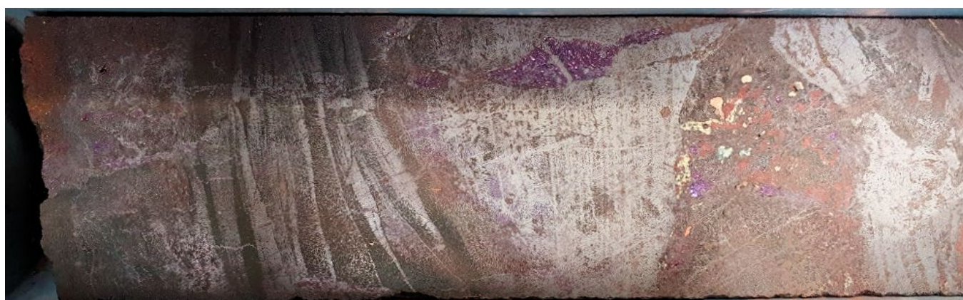
Figure 1 Photograph of NQ3 diamond drill core (nominal diameter 45.1mm) showing blebby bornite (the purple colour) sulphide mineralisation in DD21EB0018W2, from 824.64m
