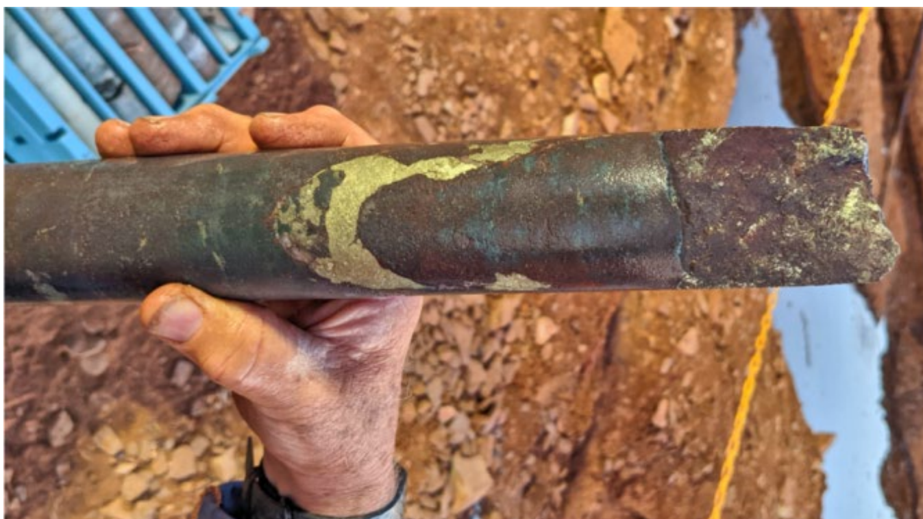
Figure 7 Massive chalcopyrite vein within a broader mineralised envelope of approximately 24.m consisting of blebs and veinlets of similar sulphides in an intensely haematized metasedimentary host rock, DD21EBD0002W1.
