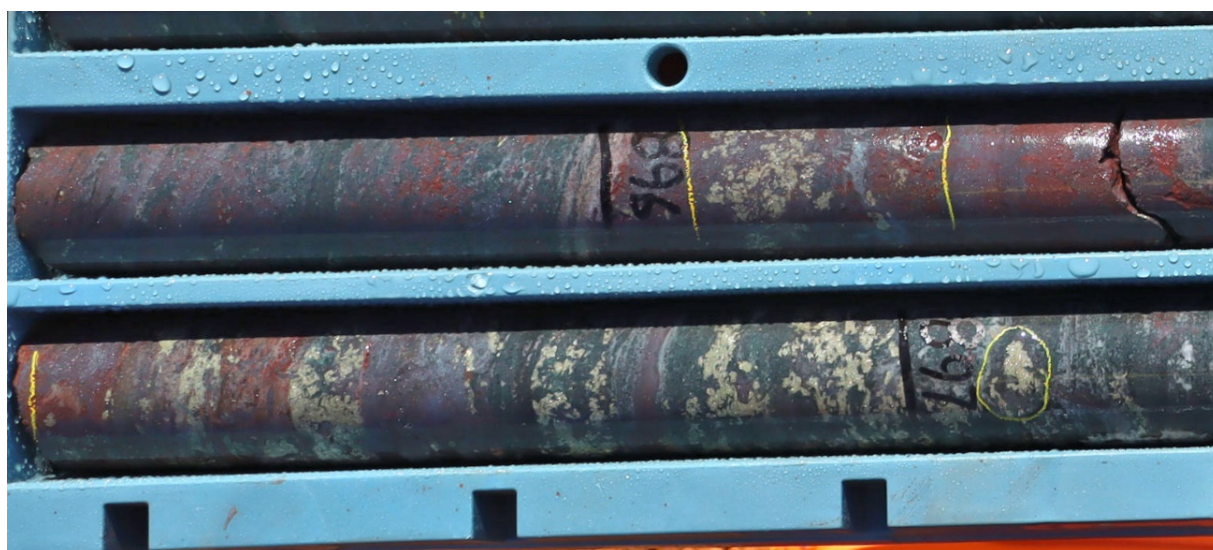
Figure 6 Mineralisation in DD21EBD0002. The sulphide assemblage includes chalcopyrite, but has a materially higher pyrite content, possibly indicative of local conditions or distance from the source of mineralisation.
