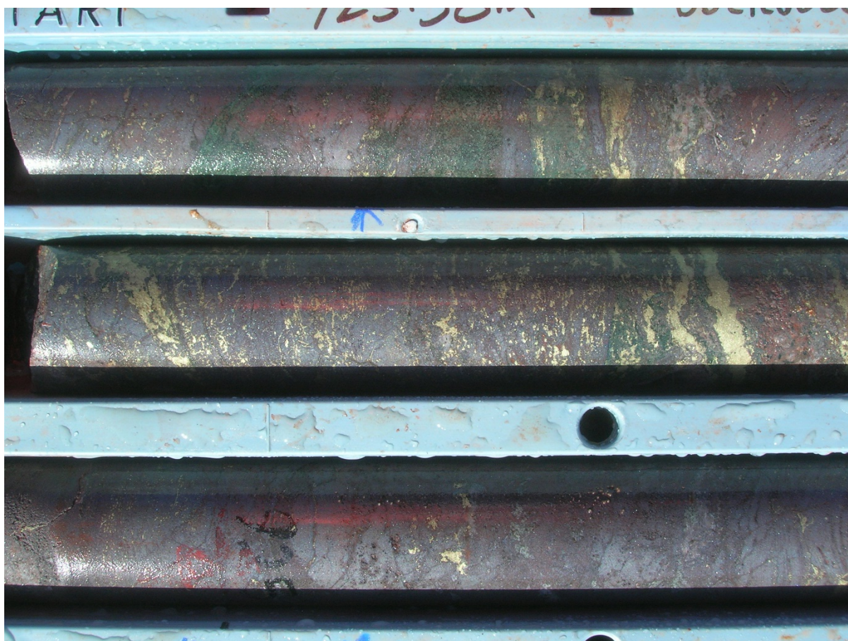
Figure 5 Chalcopyrite dominated mineralisation in the lower mineralised lode from DD21EBD0003W2.
