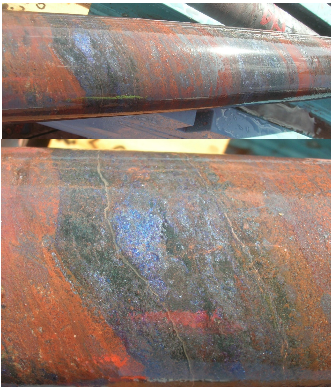
Figure 10 Bornite, covellite and chalcocite mineralisation in the upper lode of DD21EBD0003W2, including zoomed in detail shot (below).
