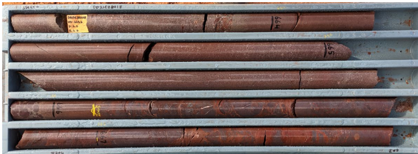
Figure 7 Core photos showing the unconformity at the base of Pandurra Fm and associated sharp transition into massive-haematite altered, brecciated Wandearah Siltstone.
