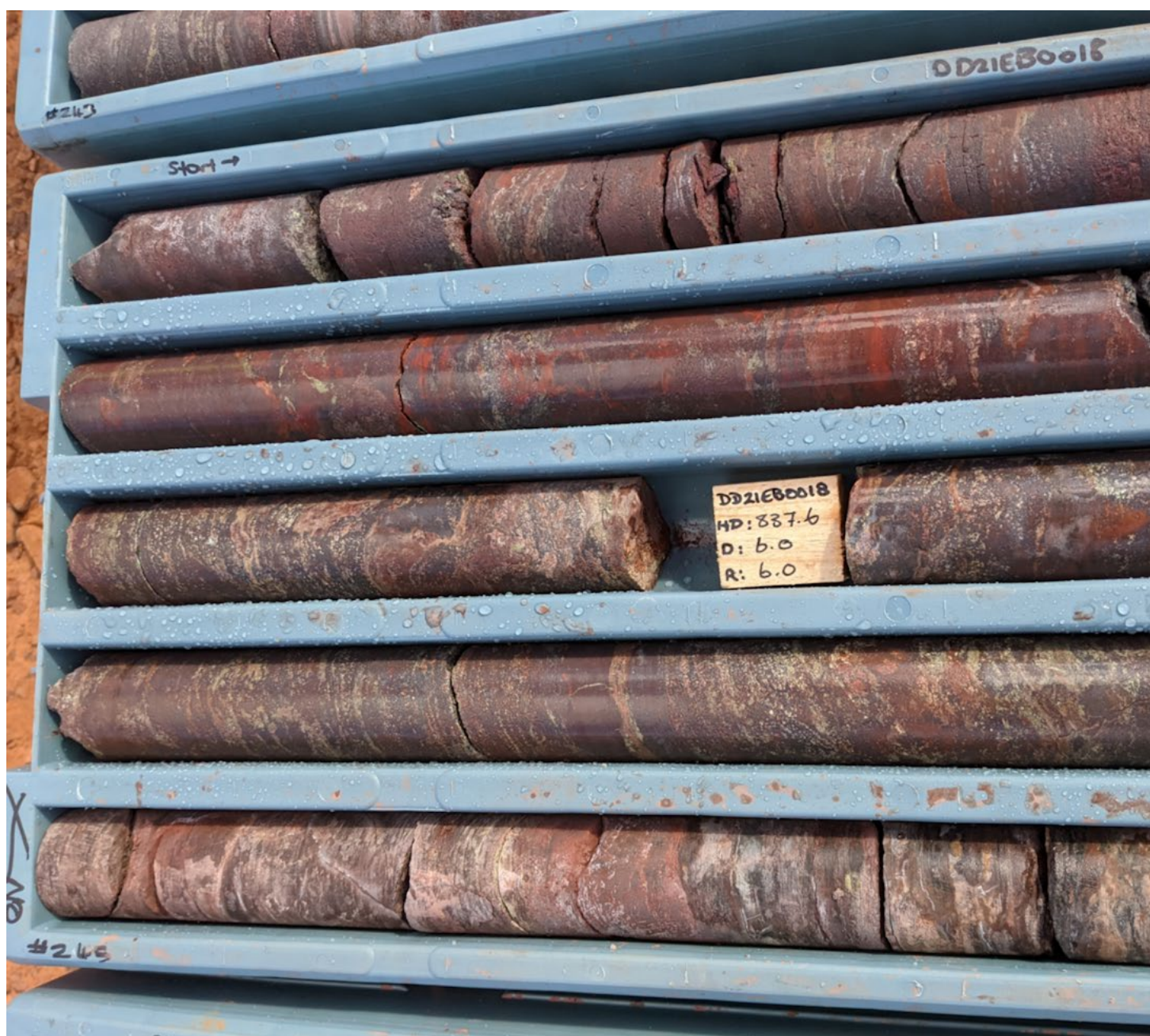
Figure 11 Typical alteration/copper sulphide pattern within the approx. 50m zone of copper sulphide mineralisation identified from approx. 797m. Chalcopyrite is the dominant copper sulphide, occurring generally parallel to remnant bedding of altered sediments, but also in small veinlets and blebs. Bornite is present only as fine disseminations in this section but is present in larger concentrations further down the hole. Note the intense patches of silica and chlorite alteration which occasionally dominate over haematite. Silica alteration becomes more intense with depth eventually dominating after approx. 850m.
