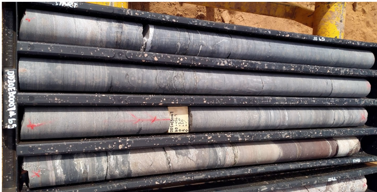
Above: Sandier mineralised Tapley Hill Fm material from eastern flank of basin. Likely represents a facies change, depositional environment may have been shallower, higher energy. Proximity to major fault encountered in hole DD20EB0002 a likely pathway for copper bearing sulphides.
