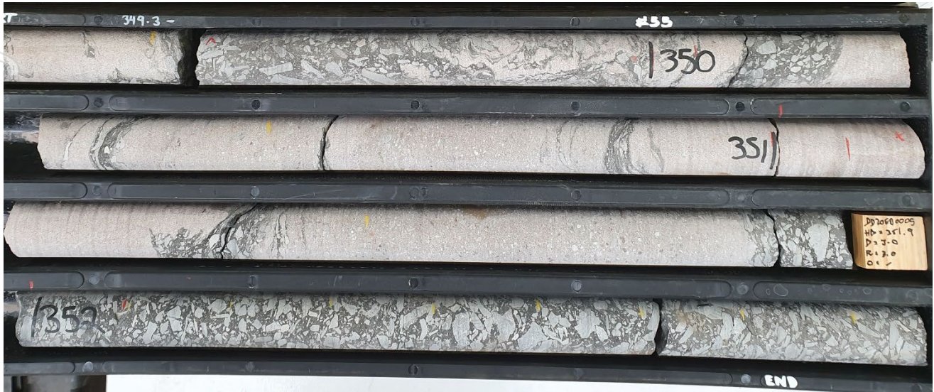
Above: Strongly brecciated intercalated Tapley and Whyalla boundary. Possible evidence for fault proximity
