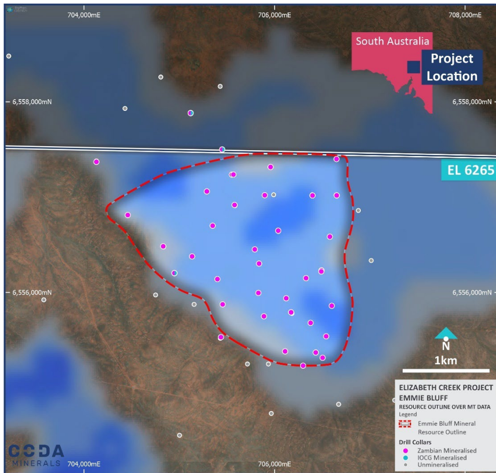
Figure 4 3D inverted ground magnetotelluric data (originally collected 2010, reprocessed 2021) showing continuity of low resistivity anomalism to the east of the Emmie Bluff Mineral Resource. The western, fault-bounded margin of the basin is well defined by contrast.
