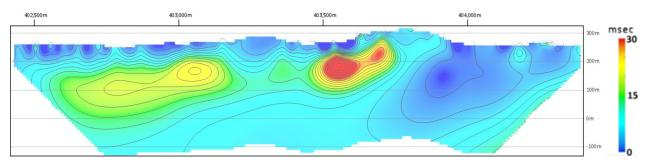
Figure 1 DDIP inversion model cross section, looking north north-east. The prominent chargeability anomaly near the centre of the survey line (up to 48 msec) is associated with the Rebound prospect. The lower intensity (up to 29 msec) anomaly in the centre west is located immediately south of Copper Weed.
