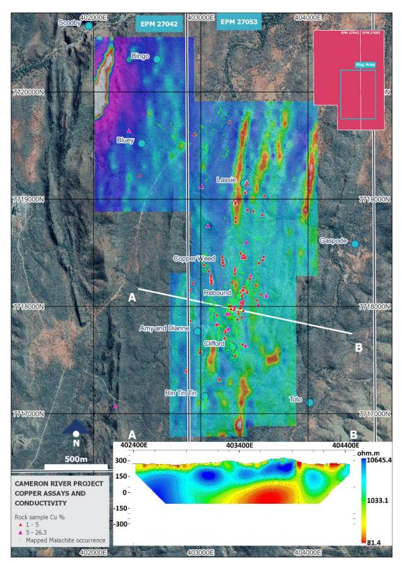
Figure 5 - Gradient Array Induced Polarisation (GAIP) conductivity grids at Copper Weed, Rebound, Bluey and Bingo, and their association with mapped malachite occurrences and copper mineralisation. Inset is the Dipole Dipole Induced Polarisation (DDIP) resistivity section (high resistivity is equivalent to low conductivity). The prominent anomaly in the northwest is under cover and remains unexplained. It has been targeted by Coda for biogeochemical (termite mound) sampling (assays pending).
