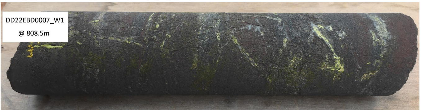
Figure 3 Chalcopyrite mineralised intensely haematised sediments, EBD7W1. Part of a mineralised sample 808.5-809.5 assayed as 0.78% Cu
