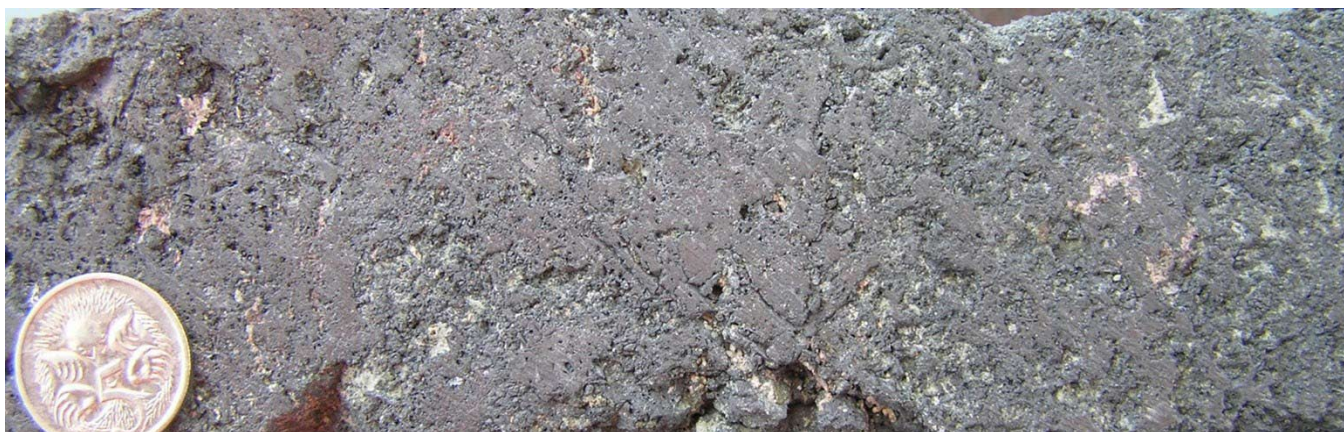
Figure 5 Typical conduit-fill texture, vuggy dark haematite, minor chlorite. Image shows NQ half core from drillhole DD21EBD0002W4, approx. depth 881.3m. 6 Coin for scale.
