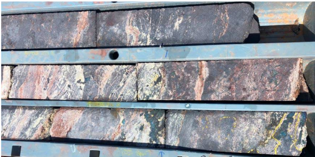
Figure 1 DD22EBD0007 mineralised material at approximately 815m. Mineralisation is dominated by bornite (abundance variable, est. between 2 and 8%) in large blebs and small veinlets, with accessory minor chalcopyrite, chalcocite and covellite (all <1%).
